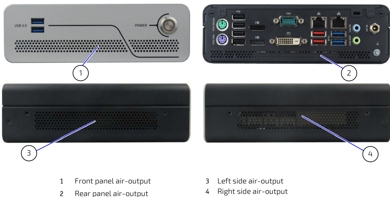
Figure 20: Air-output Ventilation Openings
