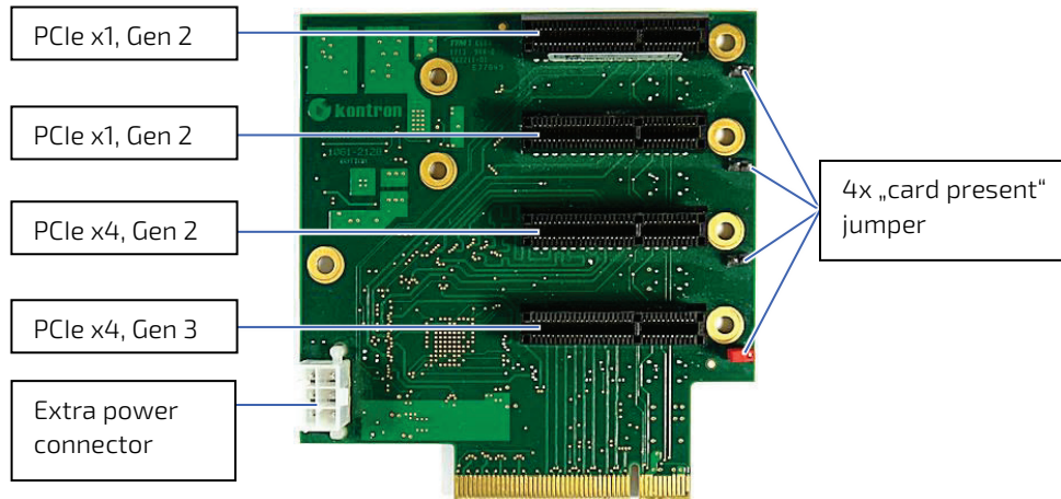
Figure 41: Riser card with 2xPCIe x4 and 2x PCIe x1 slots for KBox C-103-4
