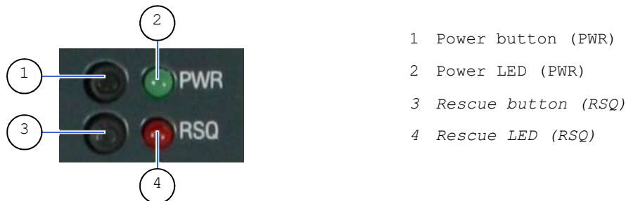
Figure 12: Detail - Power button and PWR LED/Rescue button and RSQ LED
