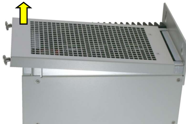
Figure 25: Removing the cover (detail of the KBox C-103-NGSF)
