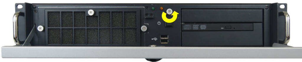
Figure 26: Loosening knurled screw on the front side
