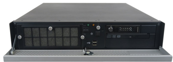
Figure 6: Desktop variant (opened front access panel)
