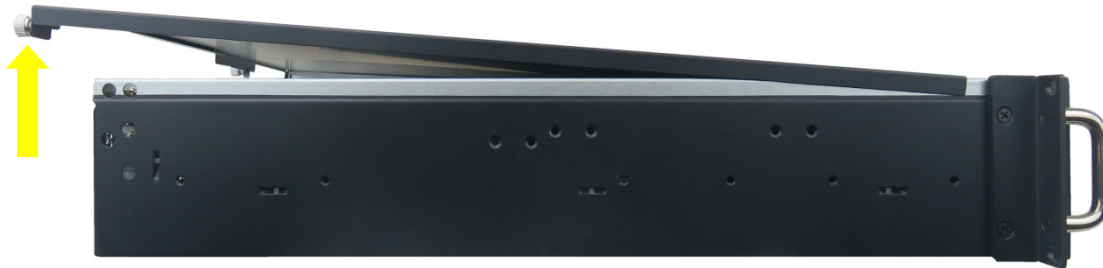
Figure 29: Removing the cover
