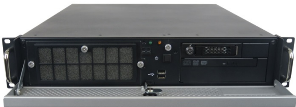
Figure 5: Rackmount variant (opened front access panel)
