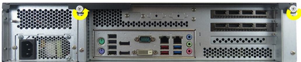
Figure 27: Loosening knurled screws on the rear side
