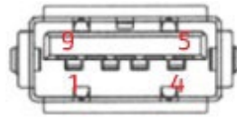
Figure 8: USB 3.2 Gen 2 Connectors CN3 - Top & Bottom (V1000 model), CN4 - Top & Bottom
