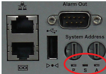
Figure 7: Status LEDs on RES2404-PTP-PoE (red circle)
