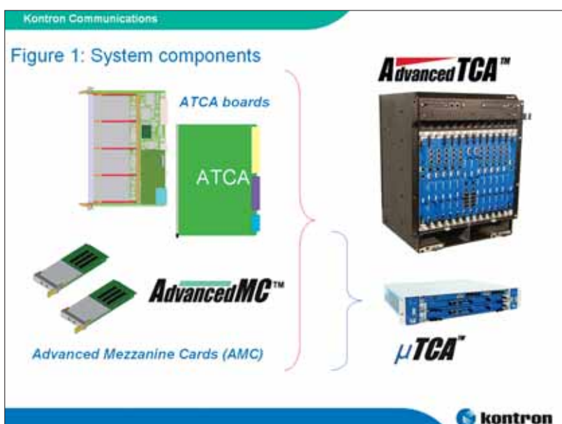
ATCA/AMC system components: The Chassis are different. They already contain 1-2 shelf managers for operating the ATCA boards and AMC as well as the fans and power supply.
